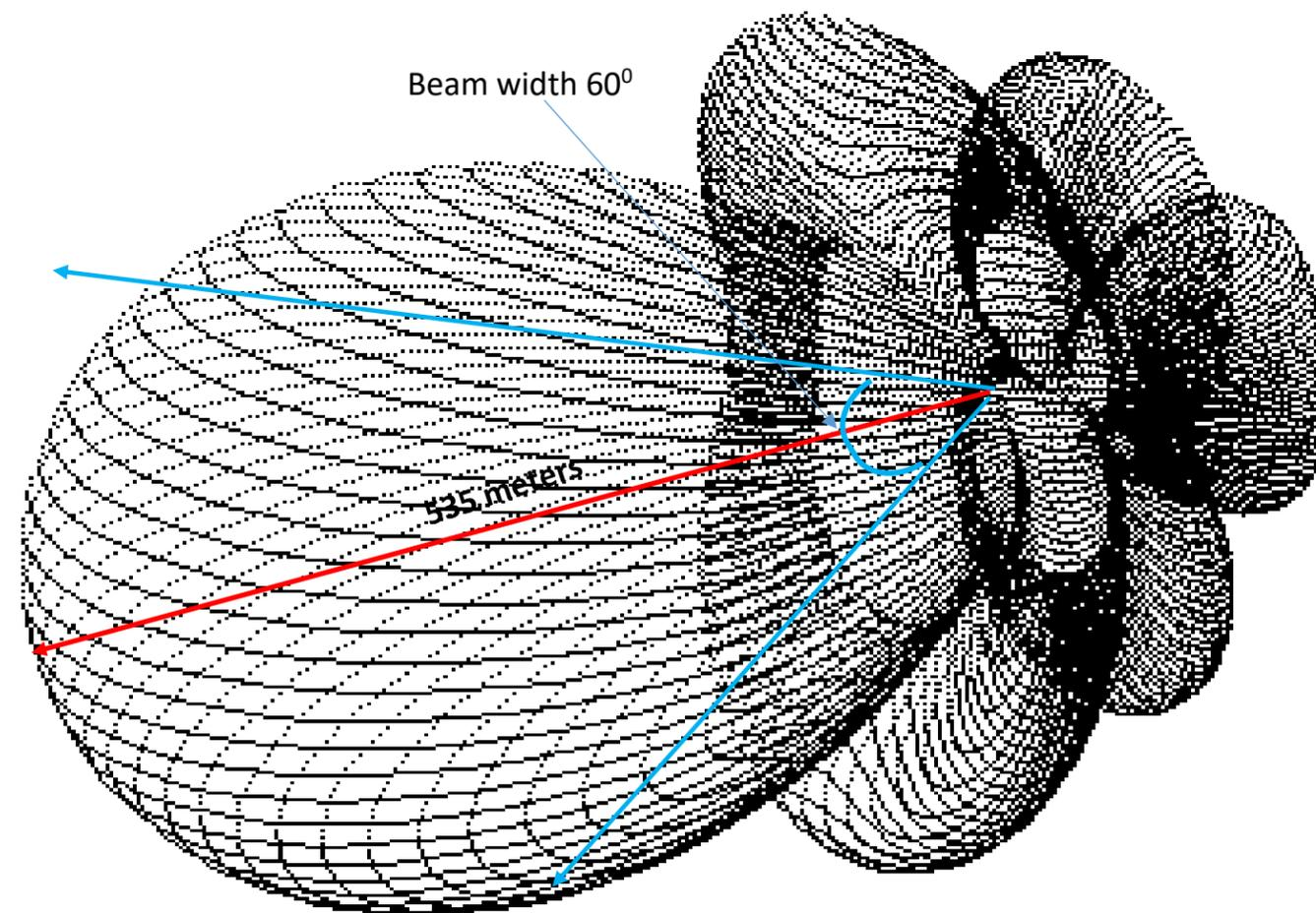
PEMF NdFeB magnet antenna radiations pattern with beam width 60° same with conventional antenna and increasing maximum range detection 535 meters with same characteristic with conventional antenna.
