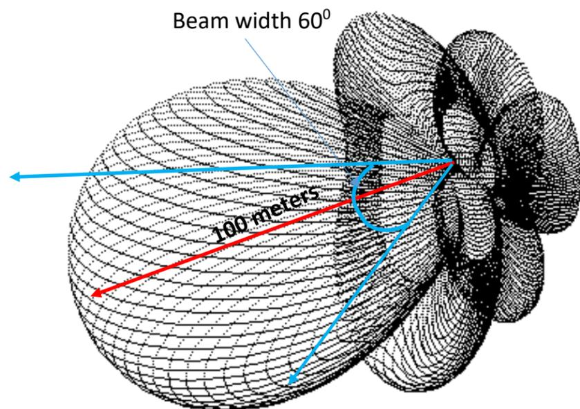
Conventional antenna radiations pattern with beam width 60° and maximum range detection 100 meters.
